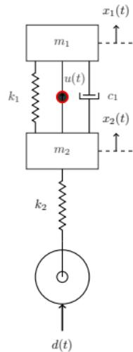
$$\begin{aligned}m_1 \ddot{x}_1 &= -k_1(x_1 - x_2) - c_1(\dot{x}_1 - \dot{x}_2) + u, \\m_2 \ddot{x}_2 &= k_1(x_1 - x_2) + c_1(\dot{x}_1 - \dot{x}_2) - k_2(x_2 - d) - u.\end{aligned}$$
